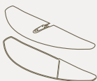
Cruiser Jet 1800 Fuselage cover 2 1 x M6 x 30mm 2 x M6 x 25mm
