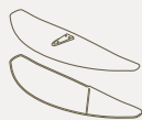
Cruiser Jet 1500 Fuselage cover 2 1 x M6 x 35mm 2 x M6 x 30mm
