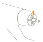
3 Insert the new Prop Pin, then position the True Glide Prop onto the shaft, ensuring engagement with the Pin.
