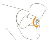
2 Remove the current Prop Pin and replace with the supplied smaller pin.
