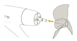
4 Seat the supplied washer into the True Glide Prop. Use the supplied tool to hold the True Glide Prop in place whilst screwing the new Nylock Nut tightly against the washer in a clockwise direction.
